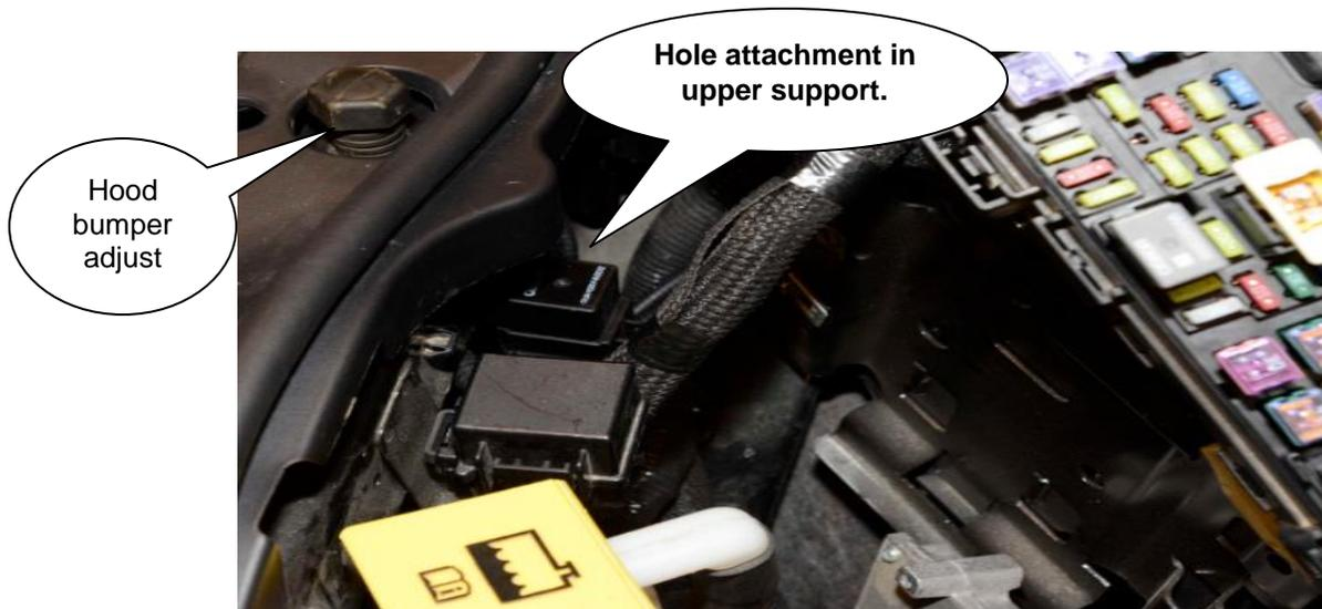
2. Unclip and roll TIPM to access the C1, 50 way black TIPM connector.
