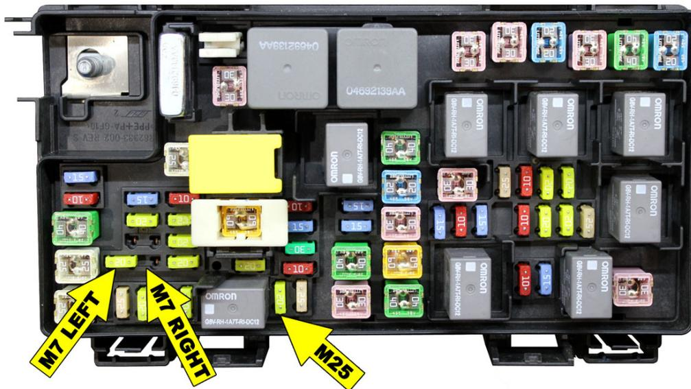
*Our cables are used with the TIPM-7 series fuse box shown at right, utilizing fuse slots M7 and M25. M7 consists of three terminals (right position provides 12 VDC when vehicle is on or off while the left position provides 12 VDC only when the key is on). One side of M25 is connected to the faulty fuel relay while the other side connects to the fuel pump. Do not use any other fuse slots to test or bypass a faulty fuel pump relay. A fuse slot diagram is shown under your TIPM lid.*
