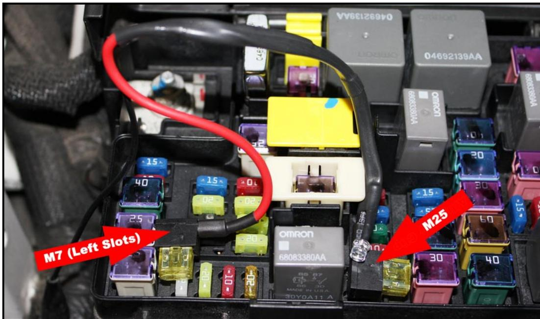
Connect one end of bypass device to M25 fuse slot, then connect other end to left slots of M7
