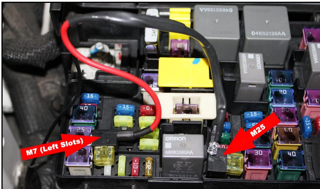
Connect one end of bypass device to M25 fuse slot, then connect other end to left slots of M7
