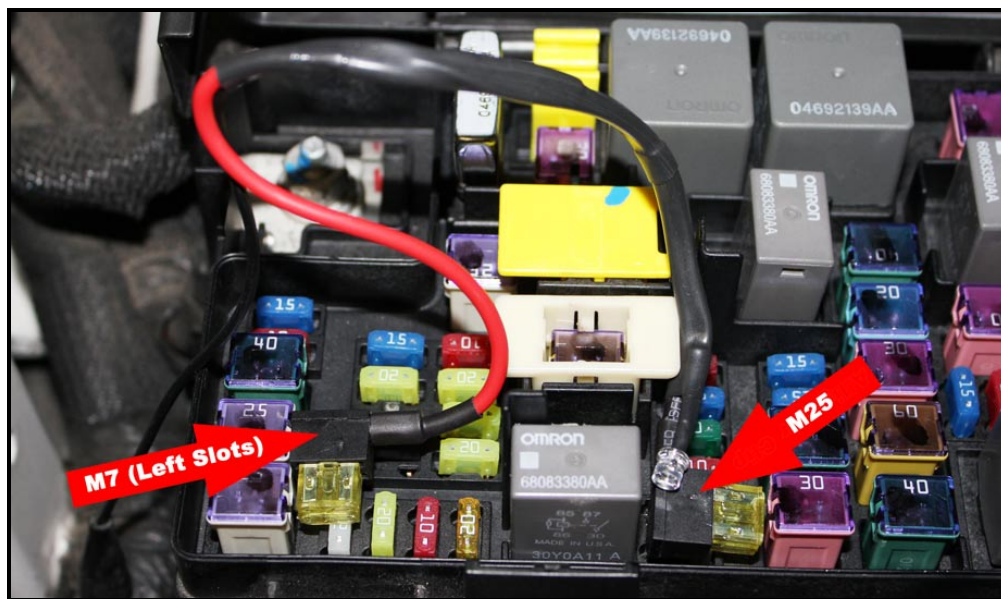
Connect LED end of bypass device to M25 fuse slot, temporarily connect alligator clip to ground, then connect bypass device to left slots of M7 for bypass mode
