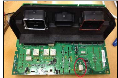
TIPM disassembled - Faulty relay shown circled in red
